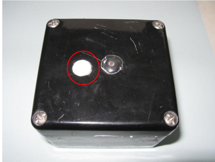
Figure 1 Example of a sample membrane mounted on the test enclosure
