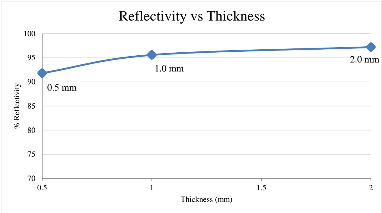
**Figure 4:** Reflectivity vs Thickness of Samples with the Same Porosity
