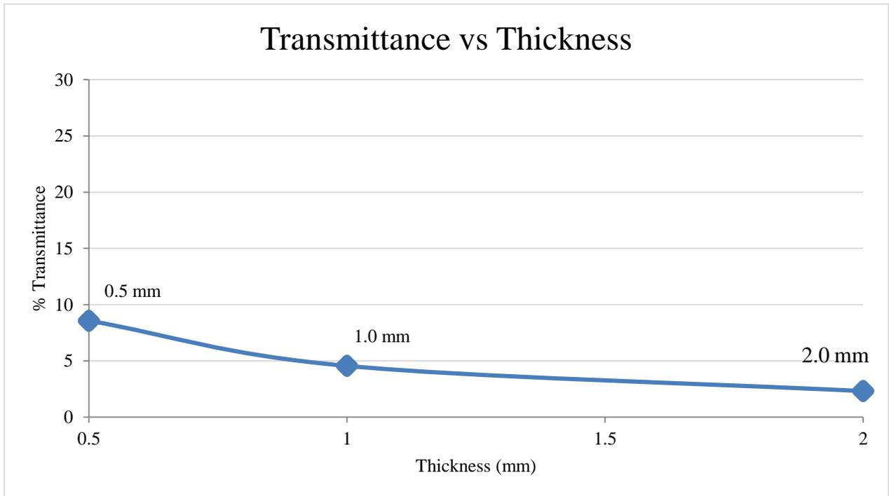
**Figure 5:** Transmittance as a function of Thickness of Samples with the Same Porosity
