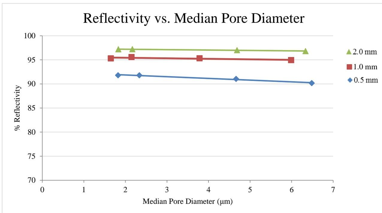
**Figure 6:** Reflectivity as a function of pore diameter.
