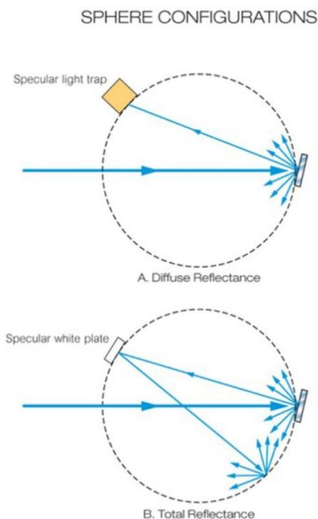
**Figure 1:** Reflectivity Test Setup.
