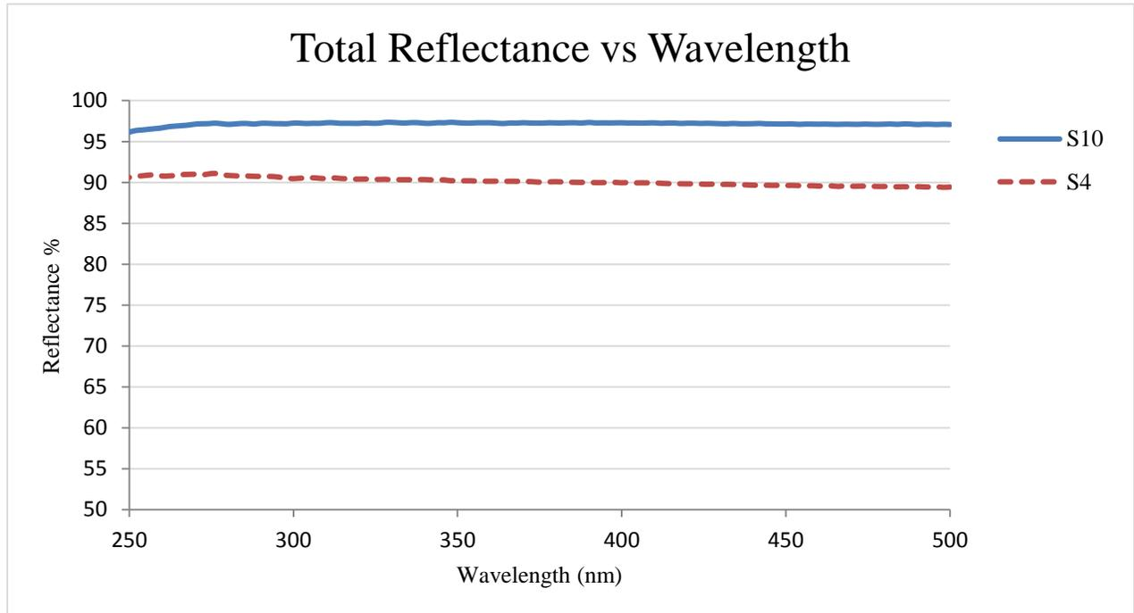
**Figure 2:** Total Reflectance. Sample 4 (Porous PTFE sheet at 0.5mm thickness) and Sample 10 (2 mm thick porous PTFE sheet) bracket the low and high UV reflectivity of the PTFE samples in the experimental set.
