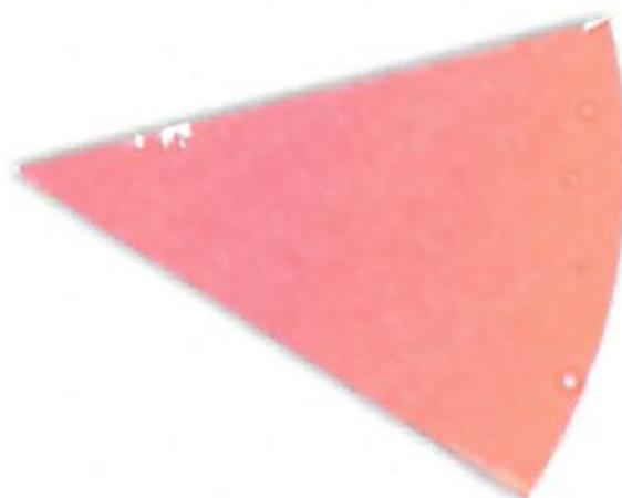
**Fig. 8.** Digital magnification of an indicator from the right side of the process challenge device after 15 min of exposure to UV-C light with polished aluminum foil as the chamber lining material.
