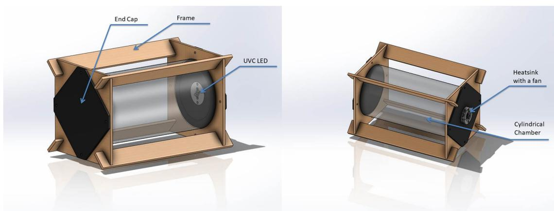
Fig. 1. Experimental test chamber construction. LED = light-emitting diode.
