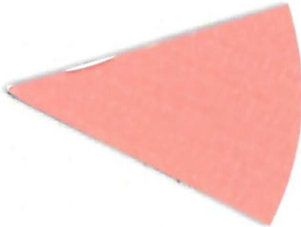
**Fig. 9.** Digital magnification of an indicator from the right side of the process challenge device after 15 min of exposure to UV-C light with PTFE as the chamber lining material.
