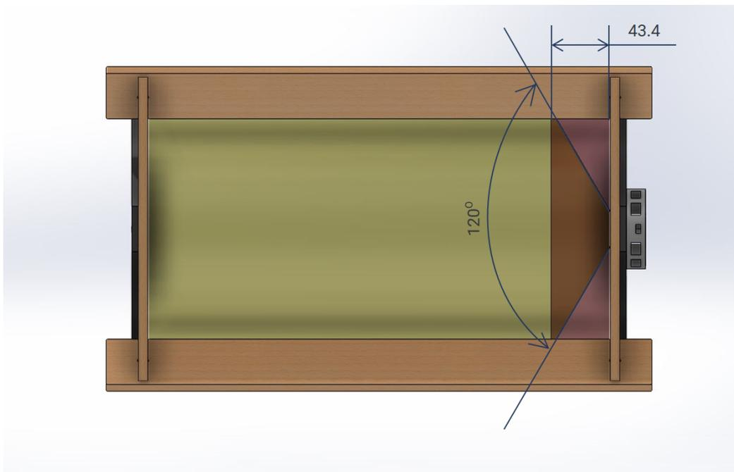
Fig. 2. Direct (yellow) and indirect (purple) light exposure zones in the chamber.
